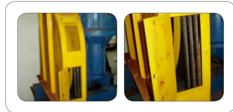
Figure 27: An example of pulley guards with a viewing window for rope inspection.
