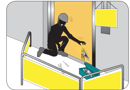
Figure 23: Equipment falling through the landing door to hoist way.
