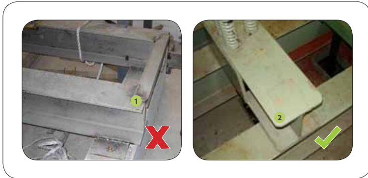
Figure 8: An example of eliminating the sharp corners of machine beams.
