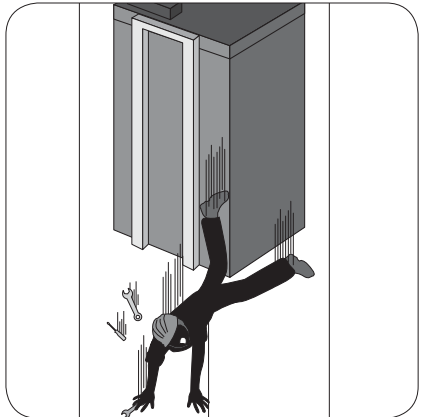
Figure 19: Falling off the top of the lift car to the bottom of the lift pit.
