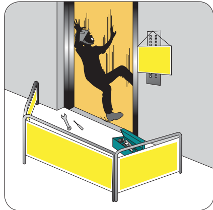
Figure 20: Falling through the opening landing door into the hoist way.
